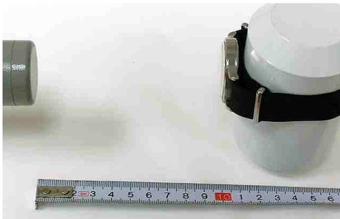
fig.9: measurement at 10 cm, dial towards detector
