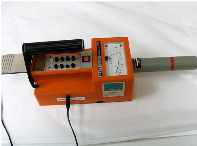
fig.5: Geiger counter for detection of radioactive contamination
