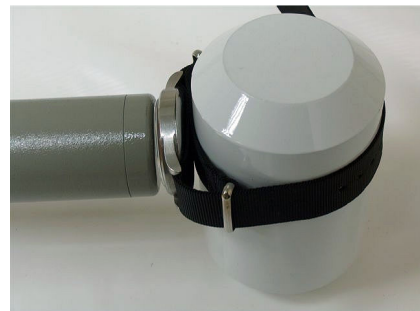
fig. 8: measurement at 0 cm, dial towards detector
