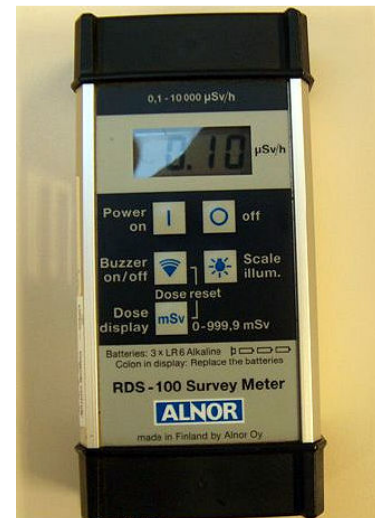
fig.6: Geiger counter to measure radiation exposure rates
