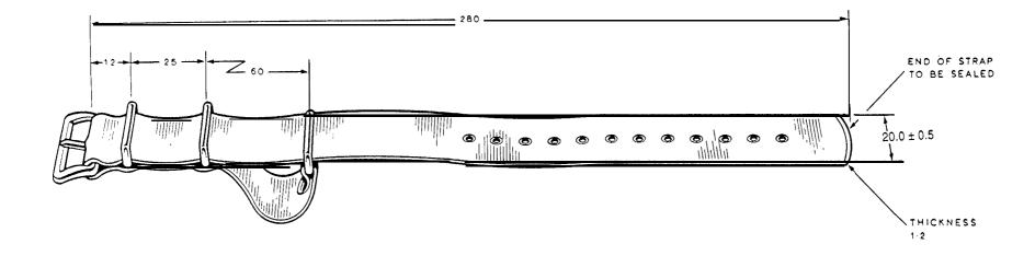
BUCKLE, PRONG, AND LOOPS — BRASS, CHROMIUM PLATED BUCKLE TO BE RECEESSED TO SECURE PRONG
